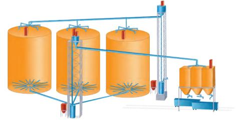
FLSmidth's Airlift<sup>™</sup> vertical conveyors and Airslide<sup>®</sup> gravity conveying systems convey alumina at a net rate of 750 mtph in a major western United States facility
