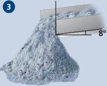
With fluidization, gravity flow can be achieved at a greatly reduced slope - of 8° or less.
