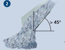
Without any fluidization, the Airslide<sup>®</sup> conveyor would need to be inclined on an angle greater than the angle of repose to establish gravity flow.
